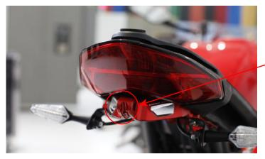
Hole caused by a high clamp.
